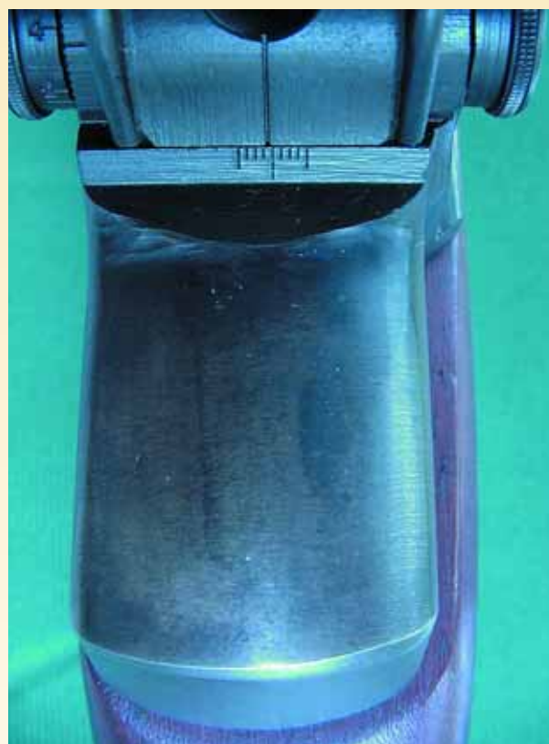
Ground, polished, and lightly blued heel of 1684.
