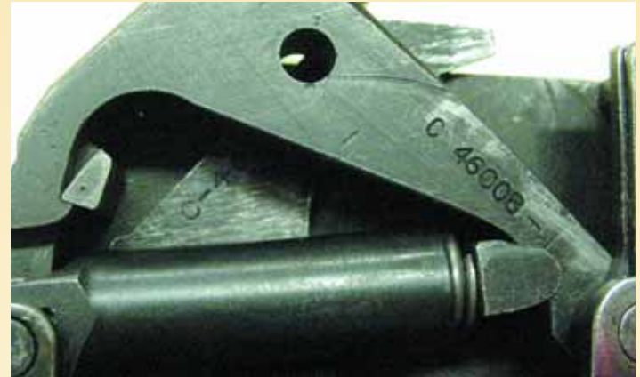
1630 hammer with -1 added by hand to the C 46008 drawing number.
