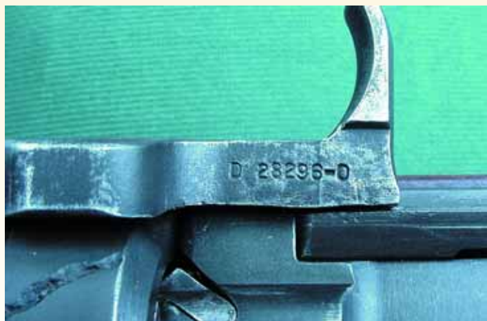
1684 Welded Seam rod. Note that the drawing number is not perfectly aligned, the D 282 is slightly higher than the 96-0. This same uneven stamping is found on the D 28296-0 rod on #81 at SANHS.
