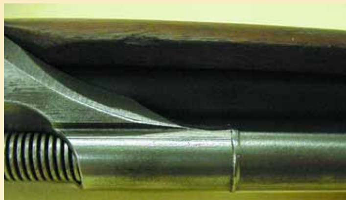
The "new" rod with tubing brazed to the handle.
