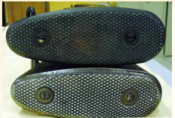
(Bottom) 1630 with worn finish and slightly flattened diamonds (Top) 1684 with sharp diamonds and all original finish.
