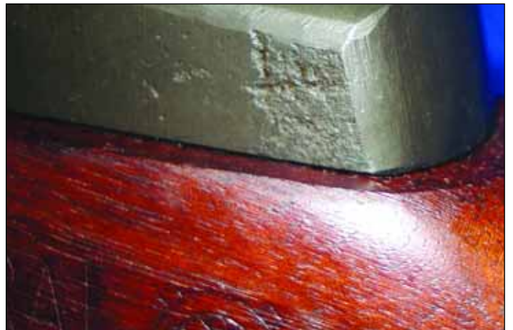
Receiver forging flaw that did not affect acceptability. These minor flaws are also found on Springfield Armory receivers, often in the area of the front receiver ring. Generally, it is the result of a forging that is slightly undersize in a small area, leaving insufficient metal for machining that area.
