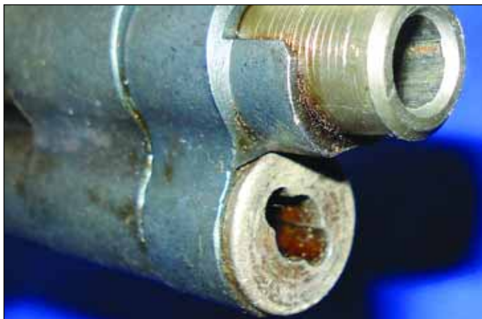
The solid lock screw is not DuLite as in earlier production, and was originally produced "in the white" with no finish. Notice, however, the pristine condition of the single slot, a good indication of little use.
