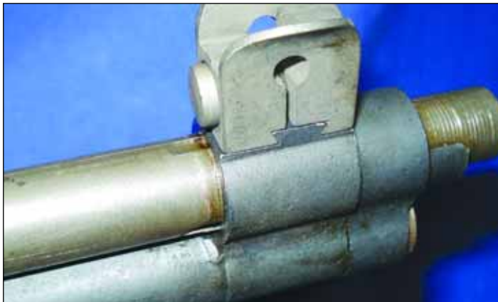
The bluish original DuLite finish is plain. The sight seal is the WRA flat face type and protrudes quite far.
