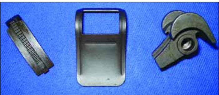
Note prick punch on the base and aperture, and partial symbol stamped on the edge of the cover.
